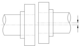
Make sure that the output shaft and the cylindrical shaft of the application are on the same axis,
