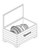
DINAMIC OIL S.p.A. gearboxes are delivered in cases, pallets, carton pallets or simple cardboard boxes, which are carefully organised to prevent movement.
