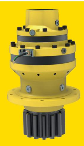
The new TD – Torque Detection system provides a digital gearbox torque signal with less than 2% of error. The integrated sensor can be inserted as an accessory into the intermediary flange and therefore will not modify standard gearbox dimensions or length.
