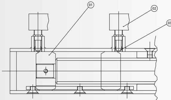
FINECORSA / LIMIT SWITCHES
